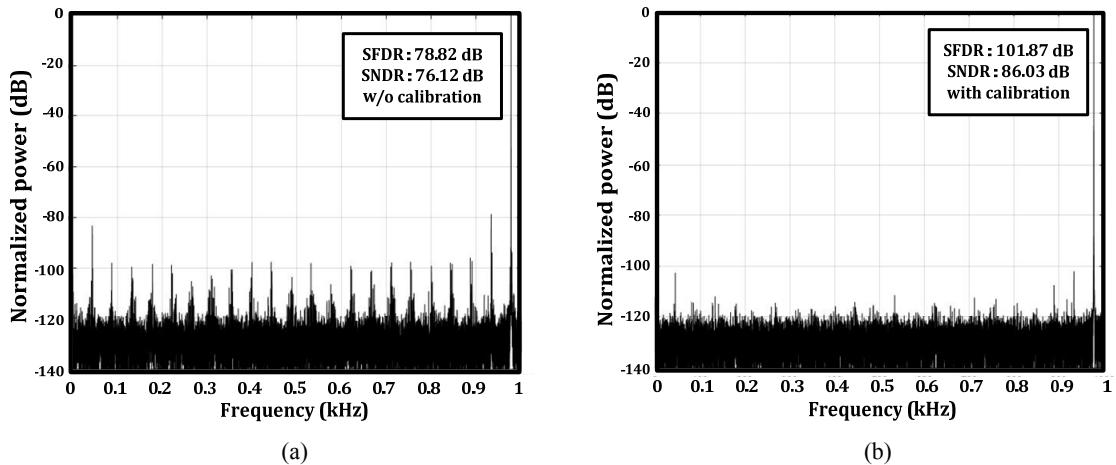
**Fig. 8.** The 65536-point FFT spectra calculated from measurements at a near Nyquist-rate input (a) without calibration, (b) with calibration.
