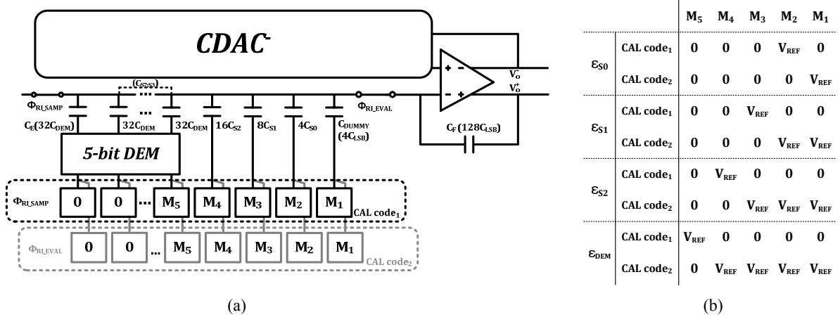
Fig. 4. (a) Circuit configurations, (b) code sets for estimation of capacitor mismatch in the calibration mode.
