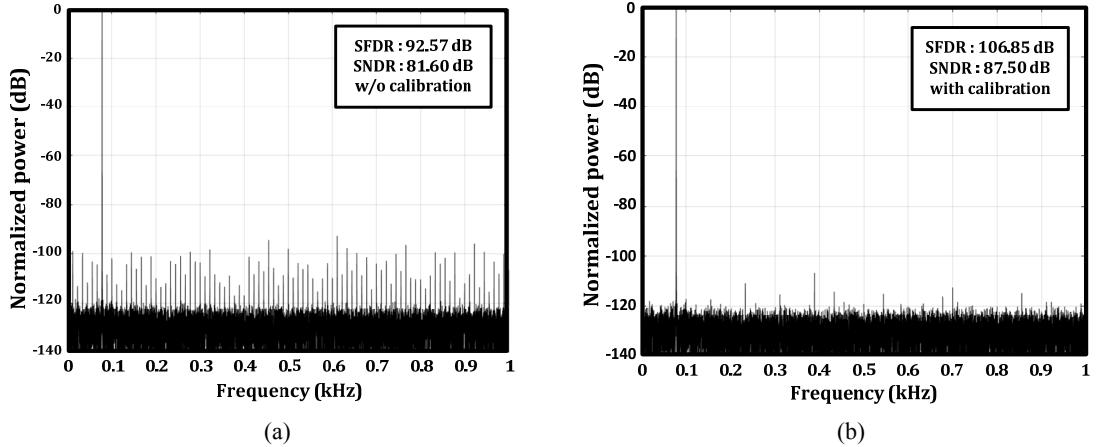
**Fig. 7.** The 65536-point FFT spectra calculated from measurement at a low-frequency input (a) without calibration, (b) with calibration.
