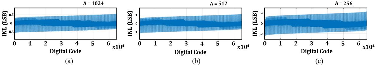
**Fig. 3.** Simulated INL with amplifier gain of (a) 1024, (b) 512, (c) 256.
