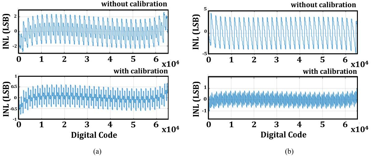
**Fig. 5.** Simulation results according to MSB capacitor mismatch applied to Gaussian statistics with standard deviation of (a) 0.02, (b) 0.05.
