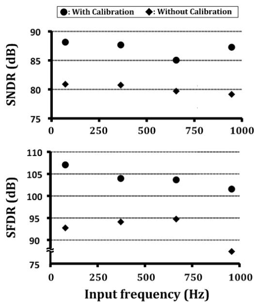
**Fig. 10.** SNDR and SFDR vs. input frequency according to use of calibration at sampling rate 2 kS/s.
