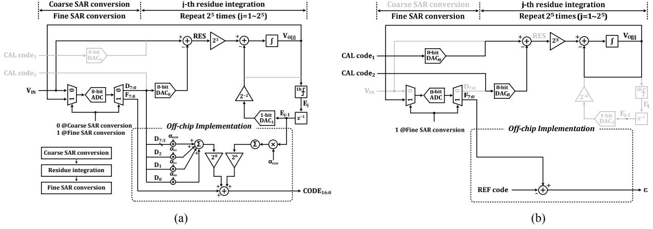
**Fig. 1.** Architecture of the proposed SAR ADC in (a) conversion mode, (b) calibration mode.
