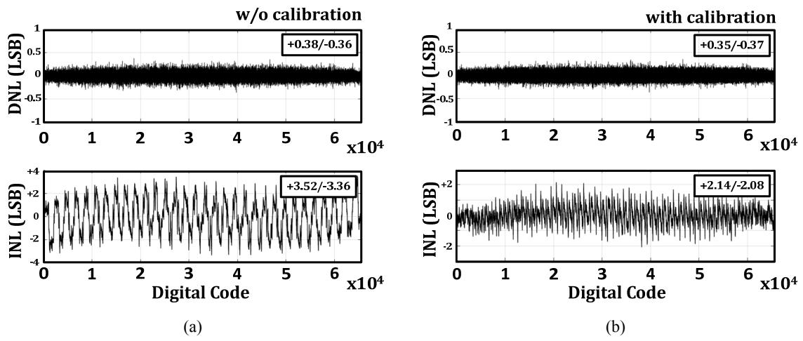
**Fig. 9.** Measured code linearity (a) without calibration, (b) with calibration at sampling rate 2 kS/s.
