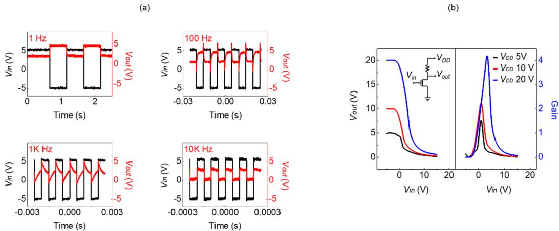
**Fig. 8.** Resistive load type inverter test by configuring the logic circuit for an a-IGZO channel layer based TFT treated with ultrasonication for 10 min (a) dynamic response characteristics based on 1 Hz, 100 Hz, 1 kHz, and 10 kHz ( $V_{DD} = 5$  V,  $V_{in} = -5$  V to 5 V); (b) results of the voltage transfer characteristic based on 5 V, 10 V, and 20 V  $V_{DD}$ .
