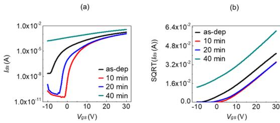
**Fig. 3.** Transfer characteristics  $I_{ds} - V_{gs}$  and square root  $I_{ds} - V_{gs}$  curves at  $V_{ds} = 30$  V in TFTs with a-IGZO channel layers treated with ultrasonication for different lengths of time (a) transfer characteristics  $I_{ds} - V_{gs}$  curves, (b) square root  $I_{ds} - V_{gs}$  curves.
