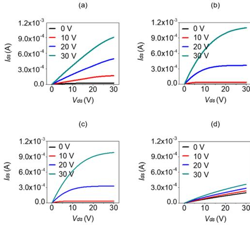
**Fig. 2.** Output characteristics  $I_{ds} - V_{ds}$  curves at four different  $V_{gs}$  levels in TFTs with a-IGZO channel layers treated with ultrasonication for different lengths of time (a) as-dep, (b) 10 min, (c) 20 min, (d) 40 min.
