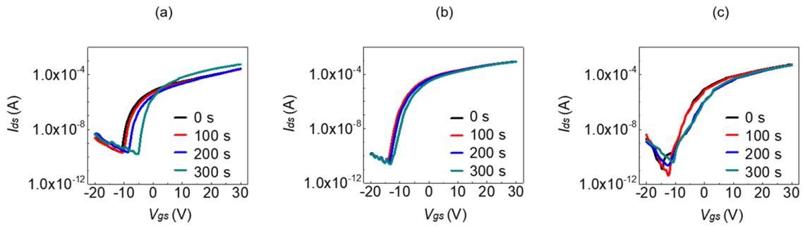
**Fig. 6.** Positive bias stress (PBS) stability of TFTs with a-IGZO channel layers treated with ultrasonication for different lengths of time (a) as-dep, (b) 10 min, (c) 20 min. The stress condition was  $V_{gs} = +20$  V.
