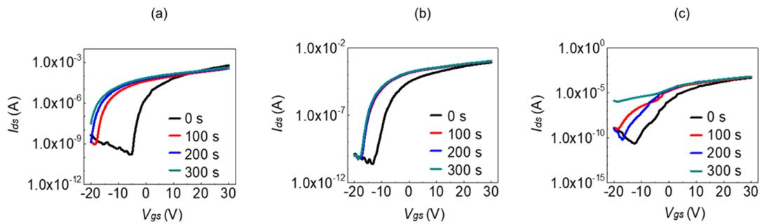
**Fig. 7.** Negative bias stress (NBS) stability of TFTs with a-IGZO channel layers treated with ultrasonication for different lengths of time (a) as-dep, (b) 10 min, (c) 20 min. The stress condition was  $V_{gs} = -20$  V.
