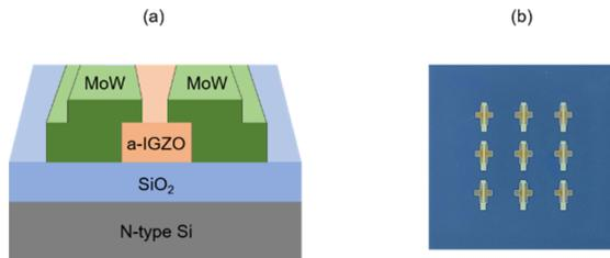
**Fig. 1.** (a) schematic diagram of a-IGZO TFT, (b) optical microscopy image of a-IGZO TFTs.
