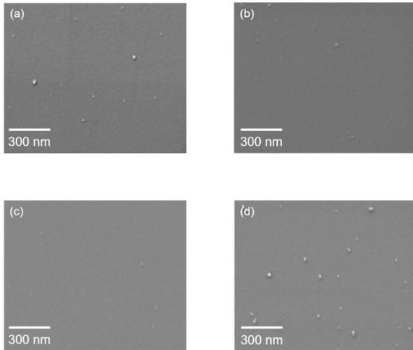
**Fig. 4.** Surface SEM images of a-IGZO channel layers treated with ultrasonication for different lengths of time (a) as-dep, (b) 10 min, (c) 20 min, (d) 40 min.
