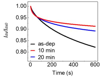
**Fig. 5.** Current stress characteristic curves for TFTs with a-IGZO channel layers treated with ultrasonication for different lengths of time: as-dep, 10 min, and 20 min ( $V_{ds} = 30$  V,  $V_{gs} = 30$  V).
