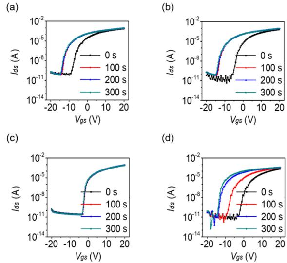
**Fig. 5.** NBS stability of TFTs with a-IGZO channel layers treated with oxygen plasma with gun-type plasma cell based on the amount of oxygen gas injected (a) as-deposited, (b) at 3 sccm, (c) at 6 sccm, (d) at 9 sccm. The stressing conditions were  $V_{gs} = -20$  V.
