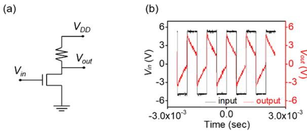
**Fig. 7.** Dynamic inverter test results from configuring the logic circuit for an a-IGZO channel layer TFT treated with oxygen plasma in which 6 sccm of oxygen gas was injected (a) schematic diagrams,  $V_{DD} = 5 \text{ V}$ , and  $V_{in} = -5 \text{ to } 5 \text{ V}$ , (b) when input frequency = 1 kHz,  $V_{DD} = 5 \text{ V}$ , and  $V_{pp} = 10 \text{ V}$ .
