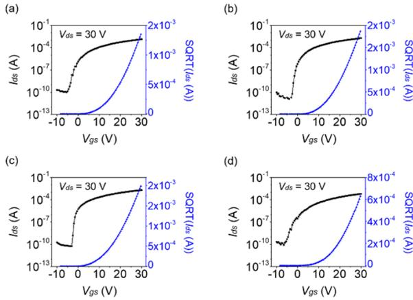
**Fig. 3.** Transfer characteristics of  $I_{ds}$ - $V_{gs}$  curves and square root  $I_{ds}$ - $V_{gs}$  with  $V_{ds} = 30$  V in TFTs with a-IGZO channel layers treated with oxygen plasma with gun-type plasma cell based on the amount of oxygen gas injected (a) as-deposited, (b) at 3 sccm, (c) at 6 sccm, (d) at 9 sccm.
