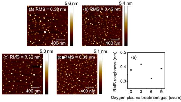
**Fig. 6.** AFM images on  $2 \mu\text{m} \times 2 \mu\text{m}$  a-IGZO channel layers treated with oxygen plasma with gun-type plasma cell based on the amount of oxygen gas injected (a) as-deposited, (b) at 3 sccm, (c) at 6 sccm, (d) at 9 sccm, (e) The change in RMS value depending on the amount of oxygen gas injected.
