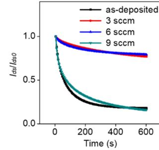
**Fig. 4.** Retention characteristic curves of TFTs with a-IGZO channel layers treated with oxygen plasma with gun-type plasma cell based on the amount of oxygen gas injected at 0 sccm, 3 sccm, 6 sccm, and 9 sccm when  $V_{ds} = 30$  V, and  $V_{gs} = 30$  V.
