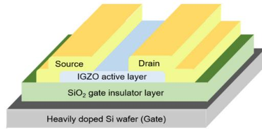
**Fig. 1.** Schematic representation of the bottom gated a-IGZO TFTs. In the device, Si is used as a gate,  $\text{SiO}_2$  is used as a gate-insulator, a-IGZO is used as an active layer (a channel layer of semiconductor), and Al is used as source and drain top electrodes.
