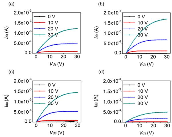
**Fig. 2.** Output characteristics of  $I_{ds}$ - $V_{ds}$  curves at four different  $V_{gs}$  levels in TFTs with a-IGZO channel layers treated with oxygen plasma with gun-type plasma cell based on the amount of oxygen gas injected (a) as-deposited, (b) at 3 sccm, (c) at 6 sccm, (d) at 9 sccm.
