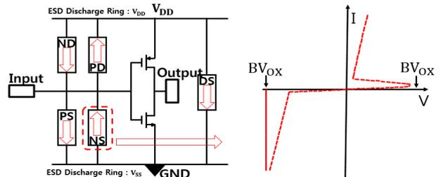
Fig. 2. ESD protection circuit composed of conventional snapback components and electrical properties of I/O clamp.
