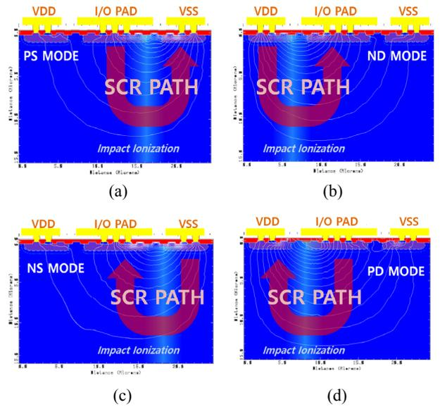
**Fig. 5.** Current path and impact ionization simulation results for I/O clamp of proposed I/O ESD Clamp (a) PS mode, (b) ND mode, (c) NS mode, (d) PD mode.
