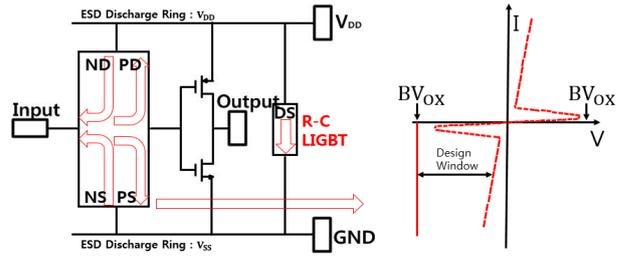
**Fig. 4.** Proposed ESD protection circuit and electrical properties of ESD clamp.
