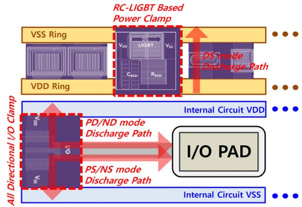
Fig. 10. Configuration of whole-chip ESD protection circuit.
