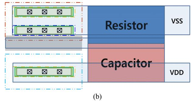
Fig. 8. Layout of proposed ESD protection circuit components (a) I/O clamp, (b) power clamp.
