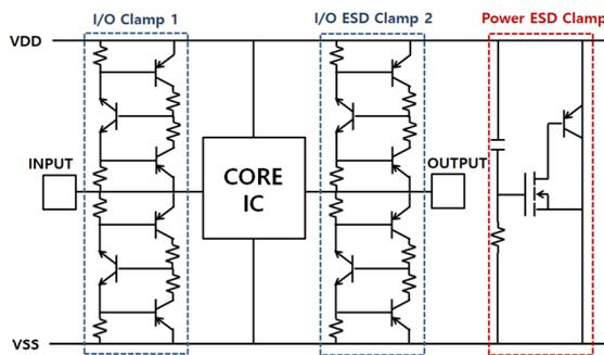
Fig. 7. Full equivalent circuit diagram of proposed all-directional ESD protection circuit with I/O and power clamps.
