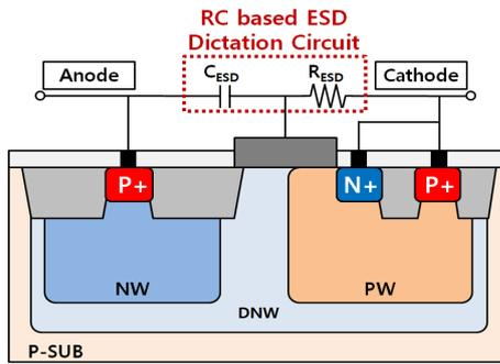
Fig. 6. Cross-sectional view of R-C LIGBT structure and layout (DS).
