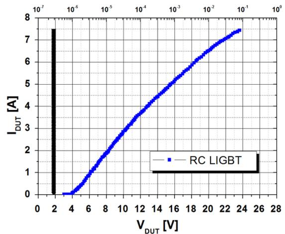
**Fig. 12.** TLP measurement results for RC LIGBT-based power clamp.
