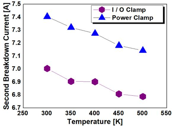
**Fig. 14.** Second breakdown current characteristic results obtained for high temperatures (300-500 K).
