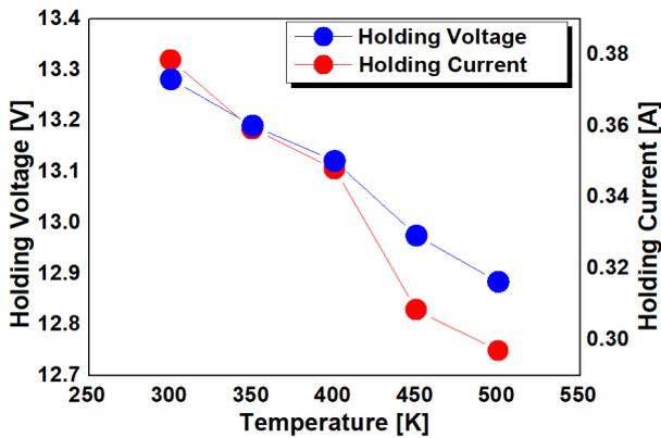
**Fig. 13.** Holding voltage and current characteristic results obtained for high temperatures (300-500 K).
