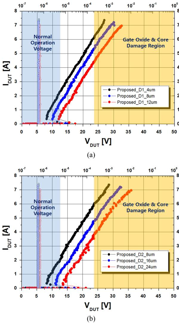
Fig. 9. Variation in holding voltage according to changes in design variables (a) D1, (b) D2.
