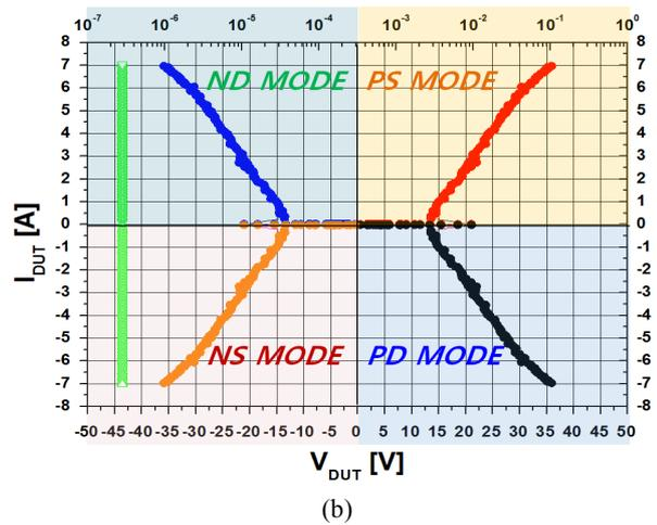
**Fig. 11.** (a) TLP measurement results for proposed I/O clamp and conventional GGNMOS and SCR circuits (PS and NS), (b) TLP waveforms for four ESD modes of proposed I/O clamp (PD, ND, PS, and NS).
