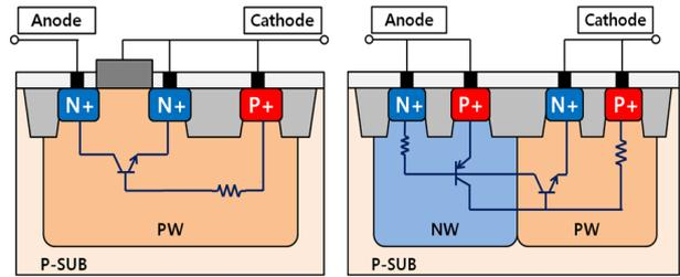
Fig. 1. Cross-sectional views of conventional GGNMOS (left) and SCR (right) ESD clamp structures.
