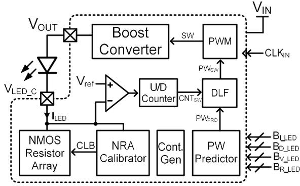
Fig. 1. Top structure of the proposed LED driver.
