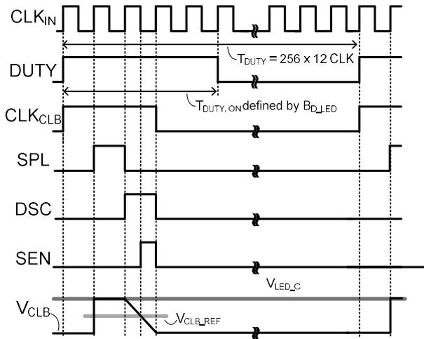
Fig. 4. Timing diagram of NRA calibrator.
