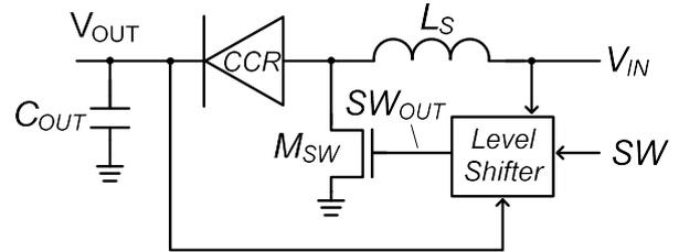
Fig. 6. Circuit diagram of the boost converter.
