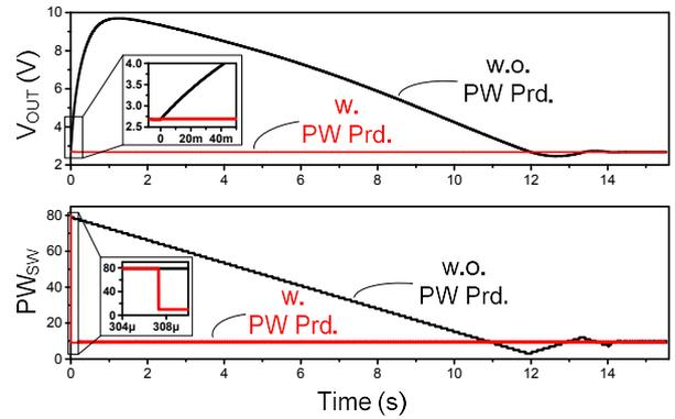
Fig. 9. Transient simulation results of boost converter.
