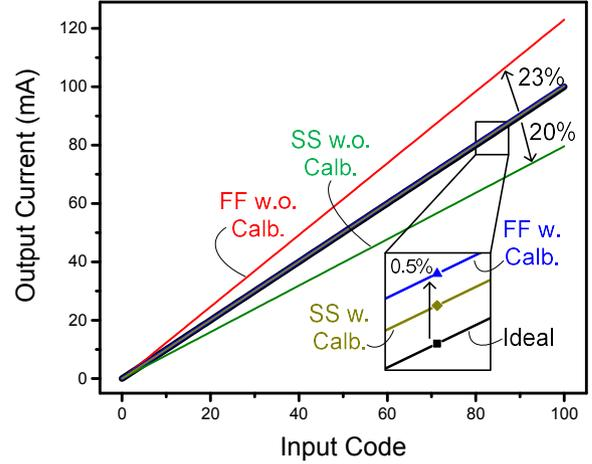
Fig. 8. Output current accuracy over process variation.
