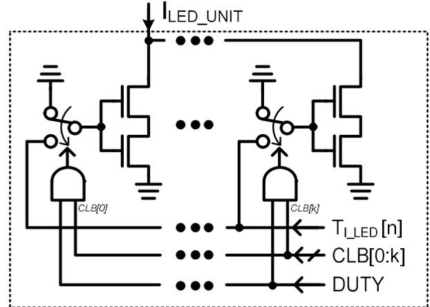
Fig. 2. Unit cell of NMOS resistor array.
