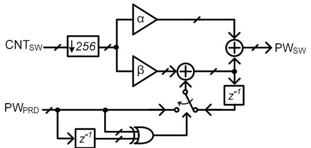
Fig. 7. Circuit diagram of the digital loop filter.
