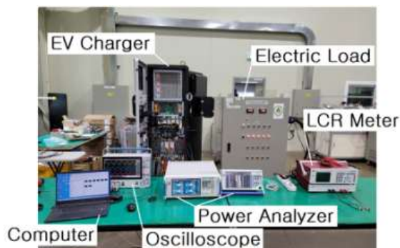
(a) Experimental Apparatus for EV Fast Charger
